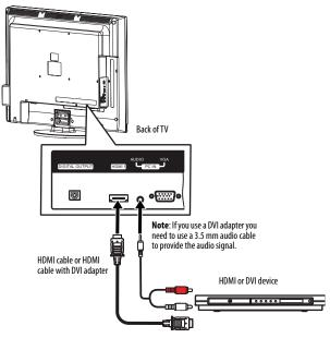
3 If you are connecting a DVI device, connect an audio cable with stereo mini plug (not provided) to the PC AUDIO IN jack on the back of your TV and to the AUDIO OUT jack on the DVI device.
